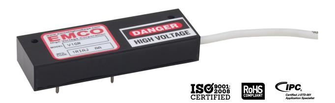
For laboratory measurement, system test point, or control loop feedback, this precision, low drift, high voltage divider provides a low voltage output from voltages as high as 25,000 VDc. The 1000:1 divider is internally compensated for your digital multimeter's 10 M $\Omega$  input impedance. Ratio tolerance is 1% and temperature drift is a low 50 ppm.
